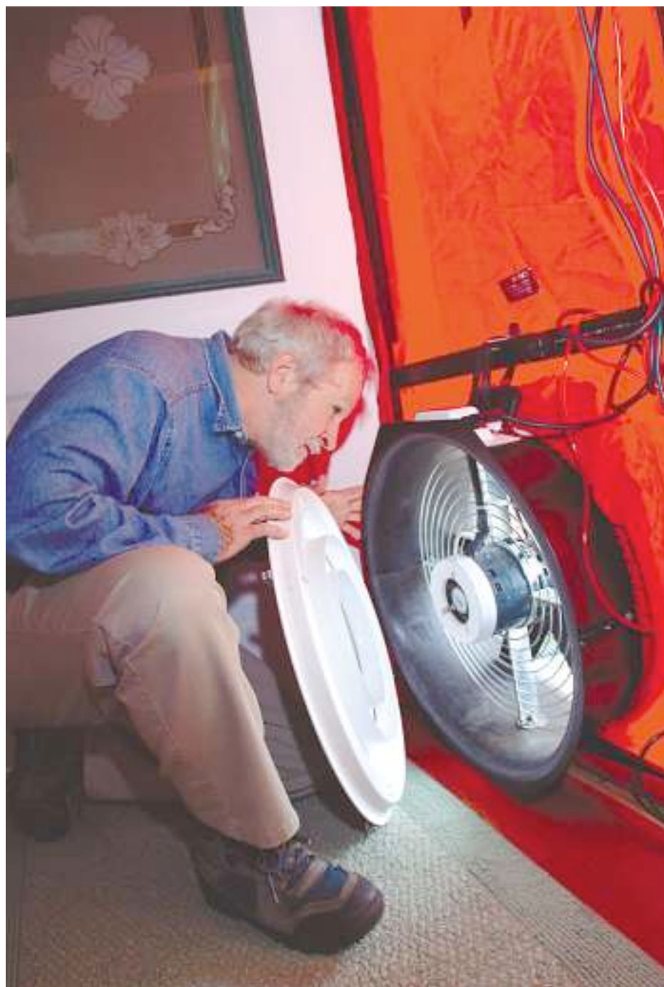
John Porterfield (left) and Earl "Cappy" Kidd (right) test a home for air leaks and heat loss using a blower door, an infrared thermometer, and a smoke puffer
